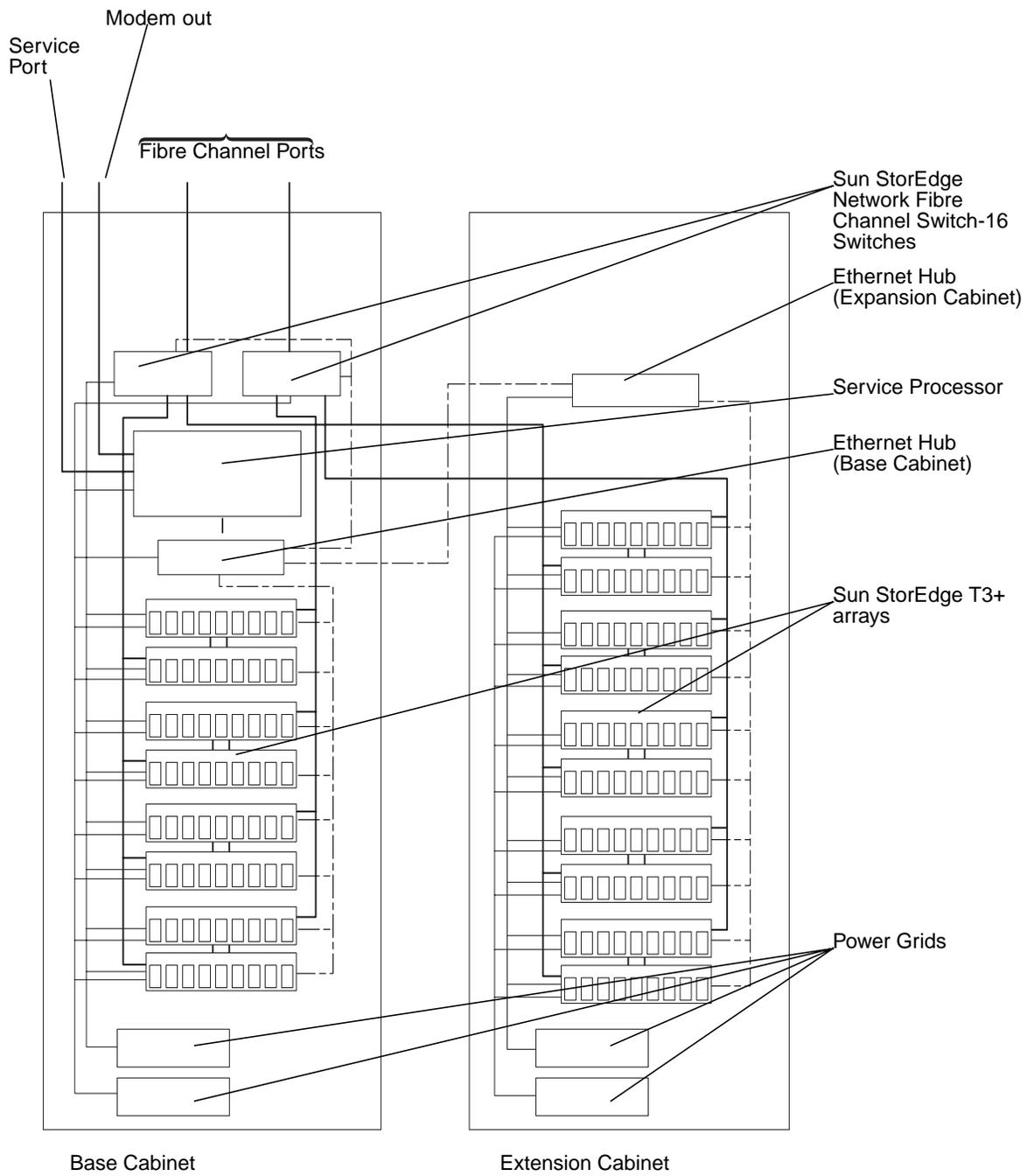
**FIGURE 3-8** Sun StorEdge 3960 Storage System Cabling
