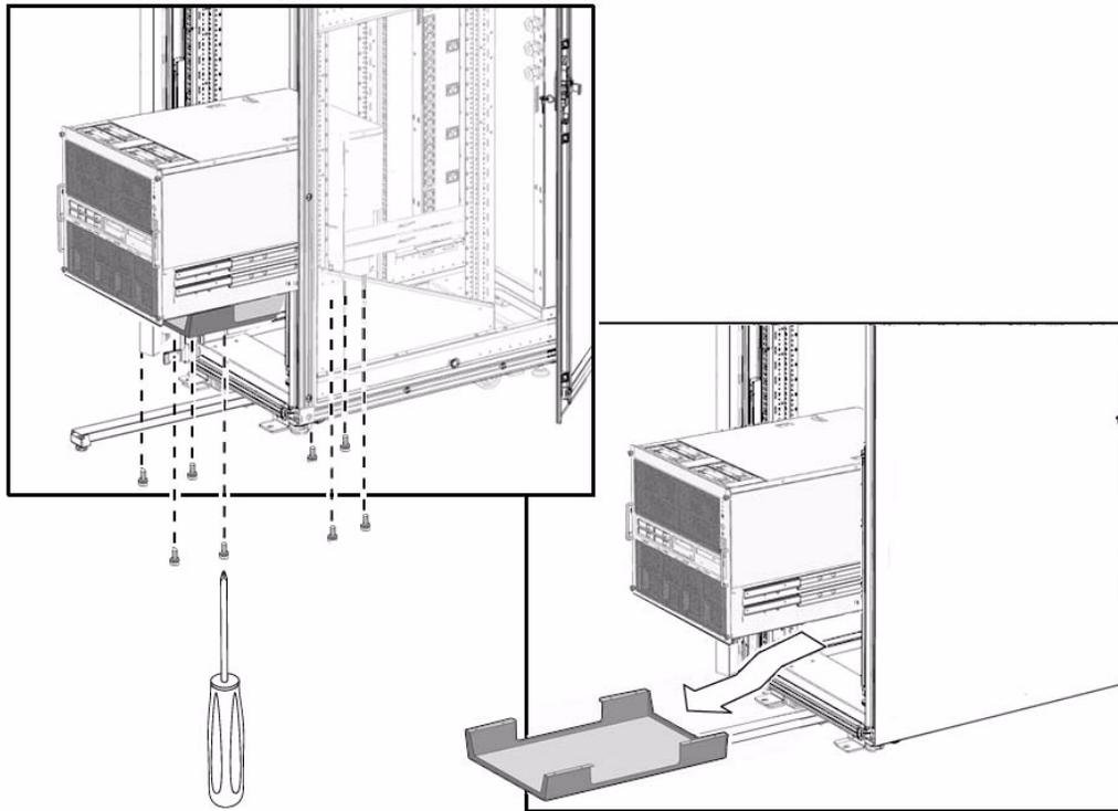
**FIGURE 6-10** Unlocking the M5000 Slide Rail
