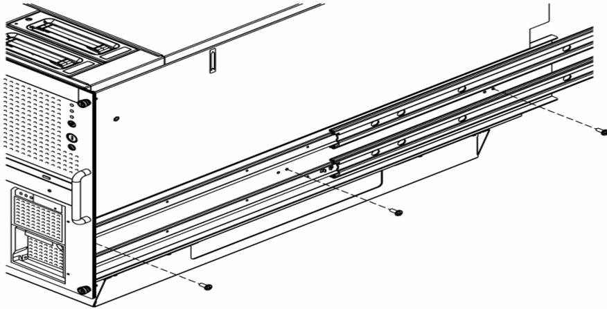
8. Remove the plinth from the bottom of the server (FIGURE 6-14).
