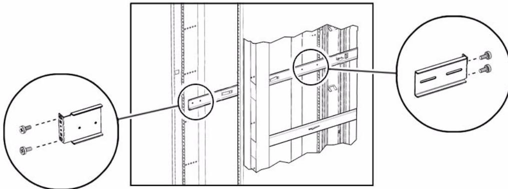
**2. Starting with the front of the rack, hook the front bracket on the rack column.**
