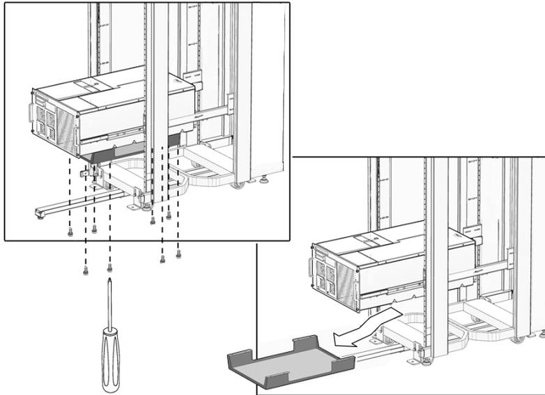
6. Withdraw the computer lifting device.
