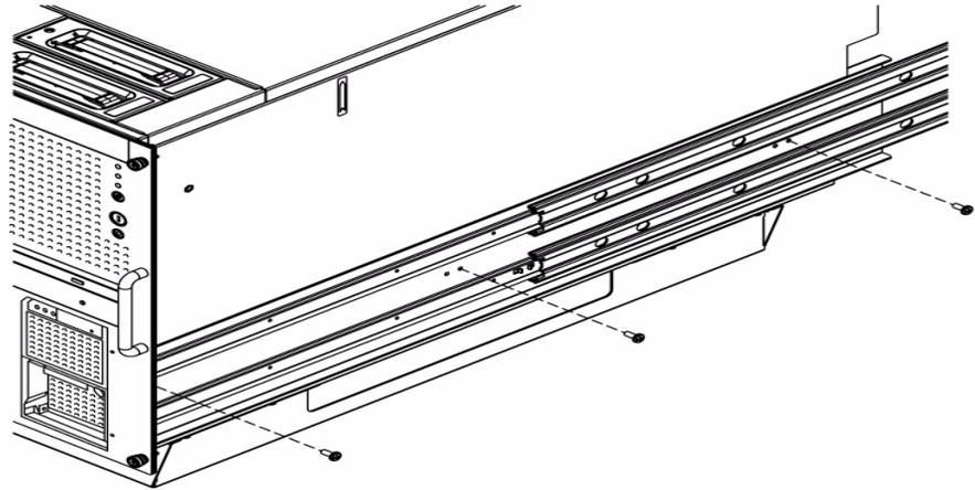
**6. Remove the plinth from the bottom of the server (FIGURE 6-9).**
