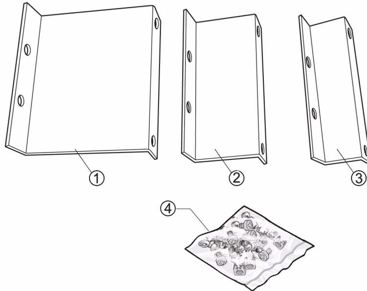
For the Sun Rack 1000/900 with the cabinet extender kit, the two large brackets are used to anchor the M5000 server to the rack prior to shipping. The two large brackets are attached through the two M5 threaded holes in the top left and top right corners at the rear of the M5000 server.
