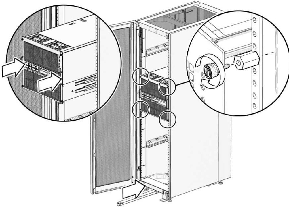
**6. Replace the anti-tilt legs to its original position.**
