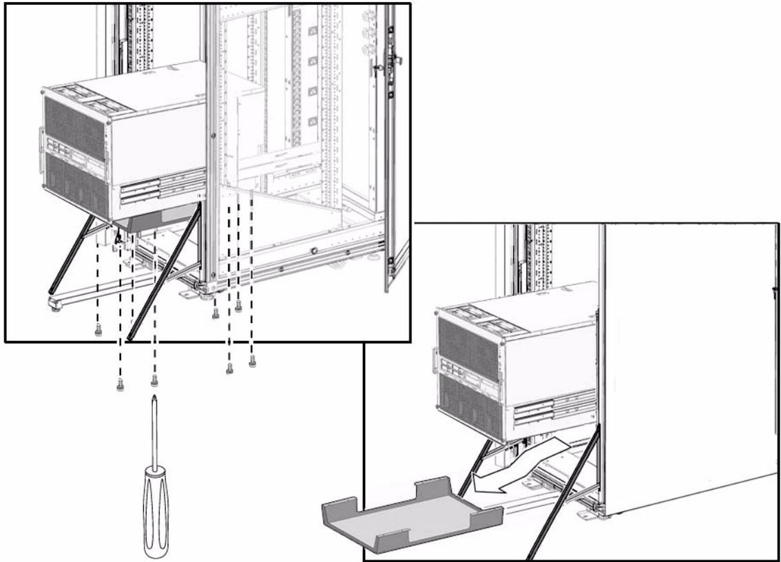
9. Withdraw the computer lifting device.
