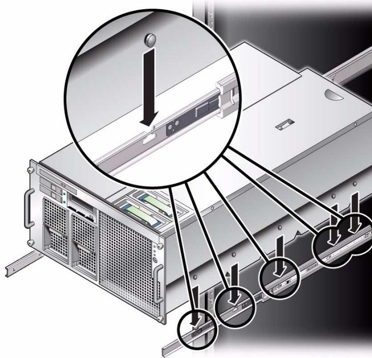
**5. Remove the plinth from the bottom of the server (FIGURE 4-10).**
