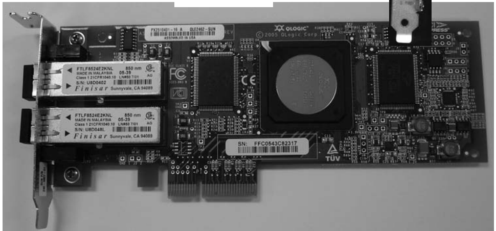
Sun StorageTek Enterprise PCI Express 4 Gb FC 單一連接埠與雙連接埠 HBA
