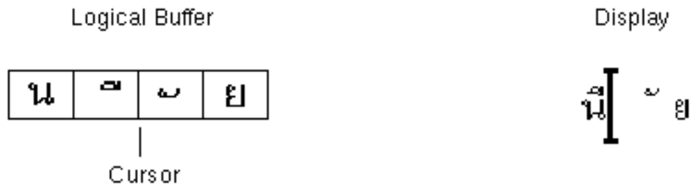
Figure D-3 Logical Buffer and Display Before Text Deletion
