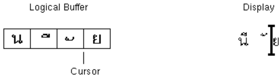
Figure D-2 Logical Buffer and Display After Text Insertion
