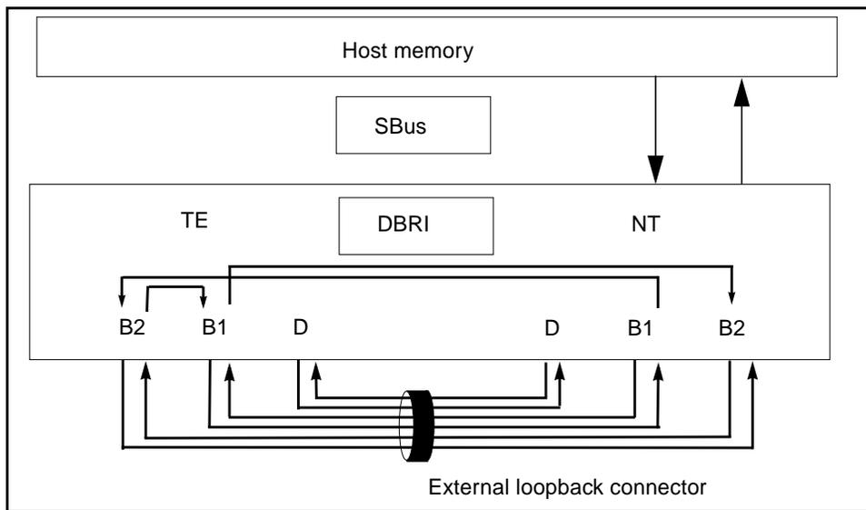
**FIGURE 24-4** isdntest Data Path Subtest
