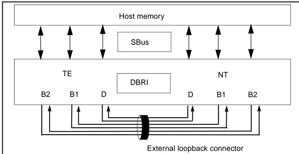
**FIGURE 24-3** isdntest Read/Write Subtest
