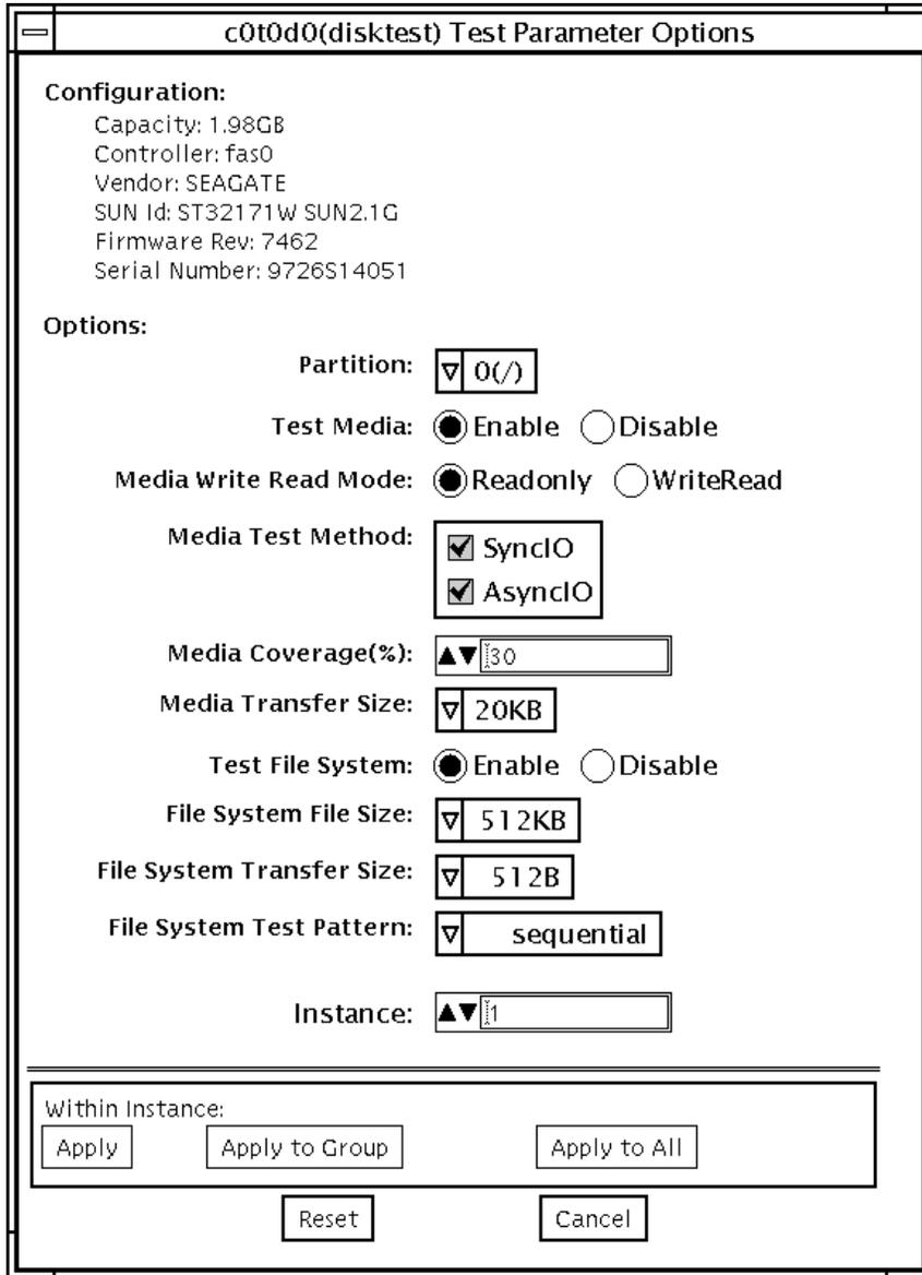
**FIGURE 10-1** disktest Test Parameter Options dialog box
