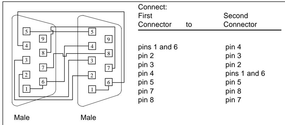
FIGURE A-14 9-Pin to 9-Pin Port-to-Port Loopback Cable
