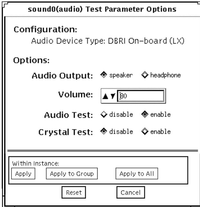
**FIGURE 4-3** audiotest Test Parameter Options dialog box for SPARCstation™ LX dbri (7) without a Speakerbox Attached
