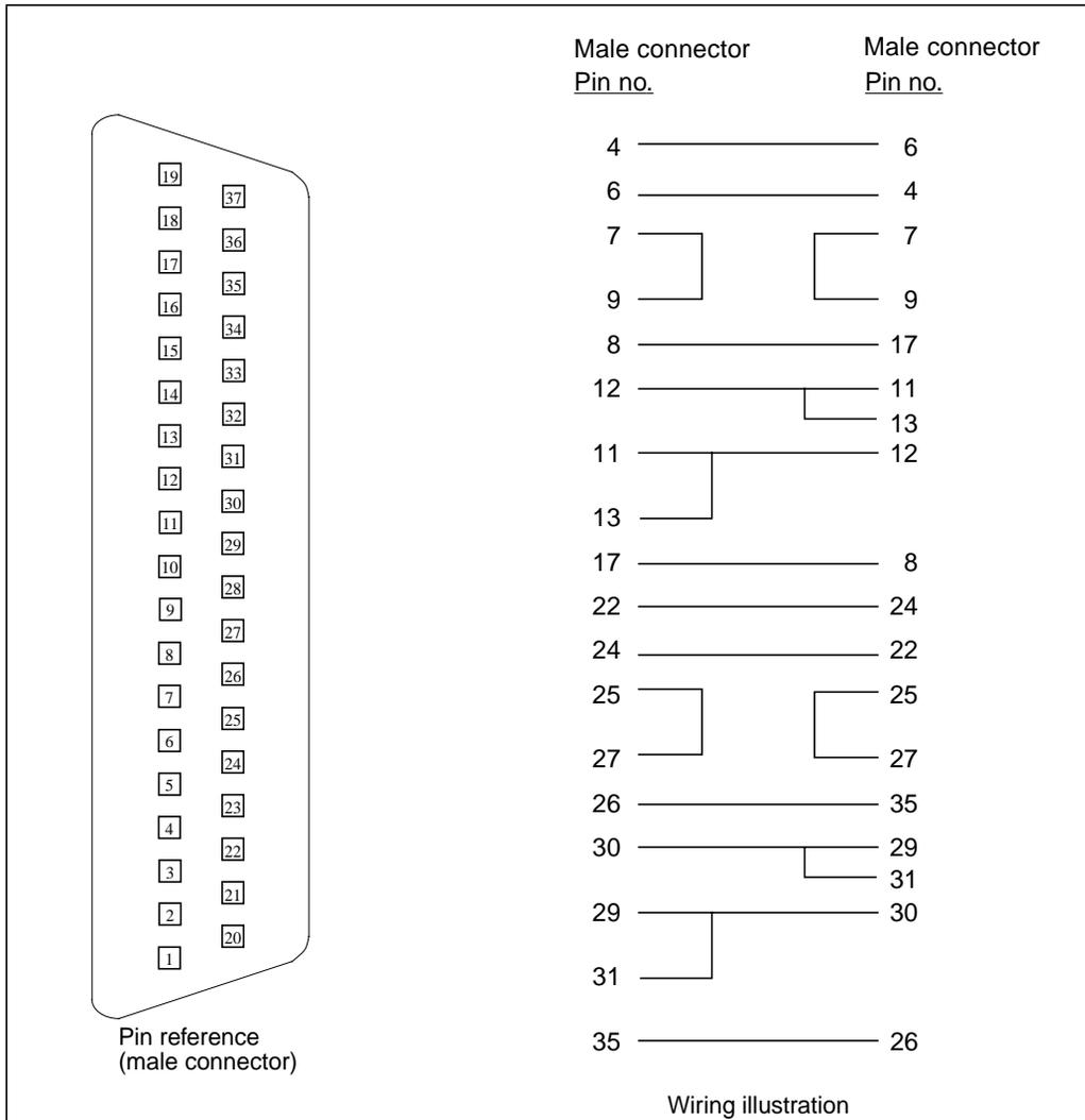
**FIGURE A-9** 37-Pin RS-449 Loopback Cable
