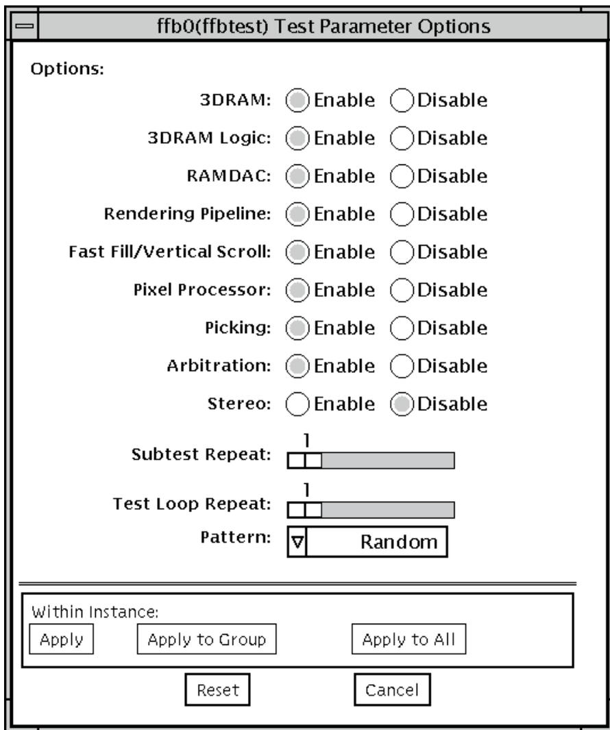
FIGURE 19-1 ffbtest Test Parameter Options Dialog Box
