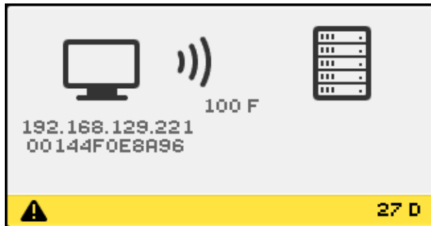
FIGURE B-12 DHCP Broadcast Failure
