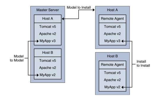
With the provisioning system you can compare one or more hosts against another host, one or more hosts against a model in the Master Server, or a host against its original configuration. The provisioning software allows you to check the entire configuration of a host or limit what is checked to a single directory.
