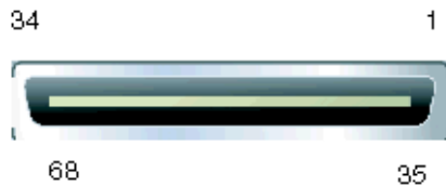
FIGURE C-1 SCSI Host or Drive Connector
