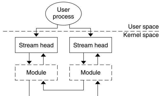
**FIGURE 6-2** Pushing Modules on a STREAMS-based Pipe
