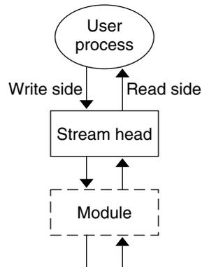
**FIGURE 6-1** Pushing Modules on a STREAMS-based FIFO
