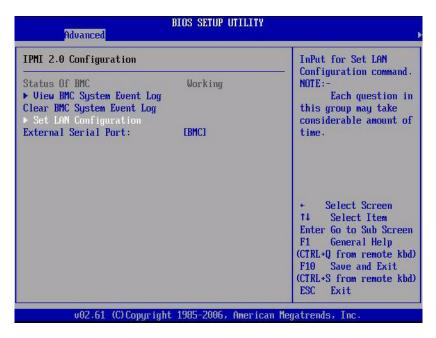
**4.** In the IPMI **2.0** Configuration screen, select the Set LAN Configuration option. The LAN Configuration screen appears.
