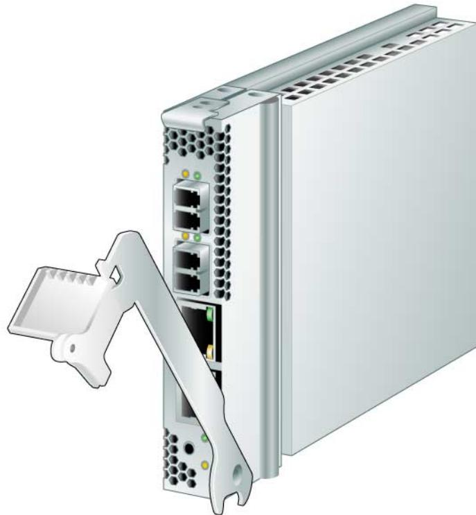
4. Insert the HBA into its slot, being careful that the tooth on the bottom of the lever does not come into contact with the chassis sheet metal during insertion.
