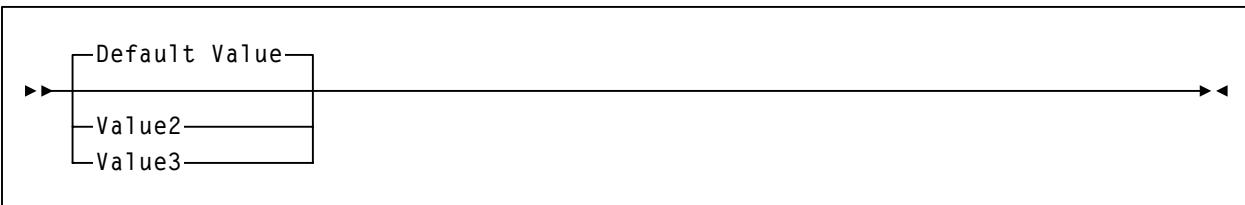
Some keyword parameters provide a choice of values in a stack. When the stack contains a default value, the keyword and the value choices are placed below the base line to indicate that they are optional, and the default value appears above the keyword line. In the following example, if the keyword is not specified with the command, the Default Value is used.
