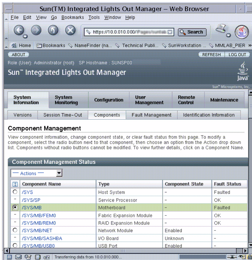
FIGURE 2-18 Enabling Components With the ILOM Web Interface
