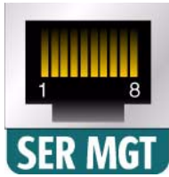
FIGURE 5-3 Service Processor Serial Management Port – Rear Panel
