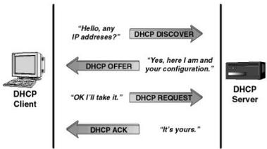
1. When booted, a DHCP client broadcasts a request, known as a DHCP Discover, looking for a DHCP server to provide TCP/IP settings. DHCP clients are found in most TCP/IP software suites for PC, Macintosh and UNIX workstations.
