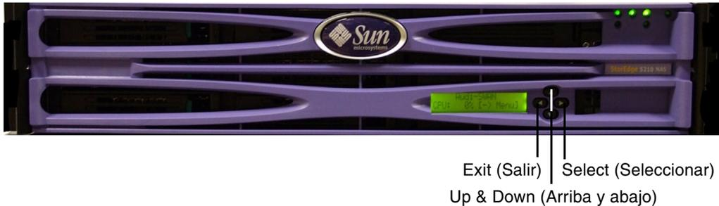
**FIGURA 2-5** Los controles del panel de LCD
