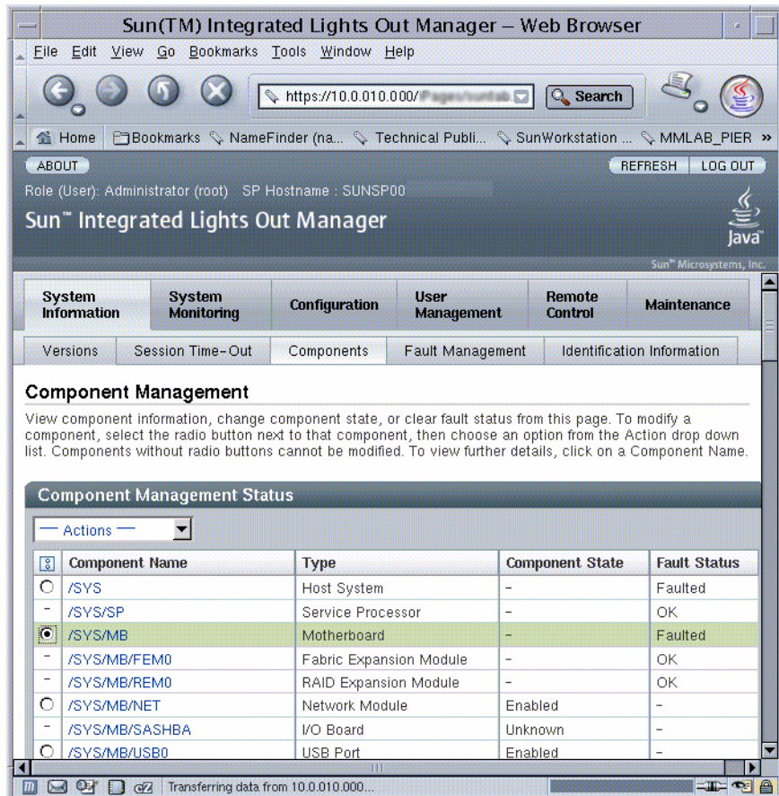
FIGURE 2-16 Enabling Components With the ILOM Web Interface
