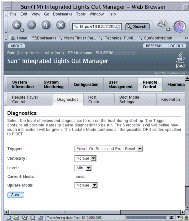
FIGURE 2-14 Setting POST Parameters With the ILOM Web Interface
