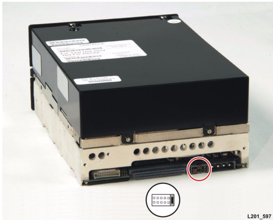
Figure 1-16. Quantum Certance Drive Terminating Power Jumpers
