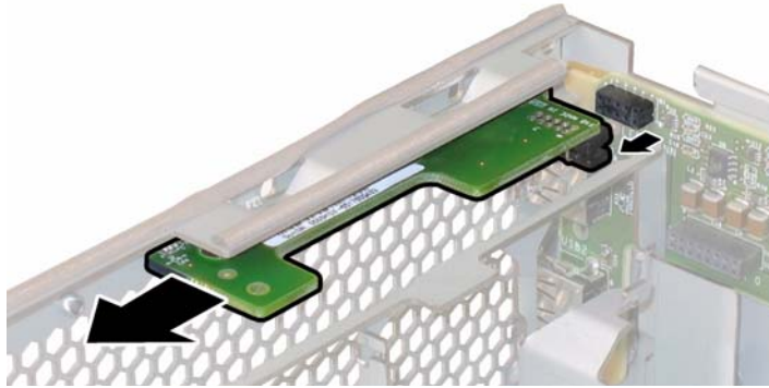
FIGURE 12-10 Removing the Front Panel Indicator Board
