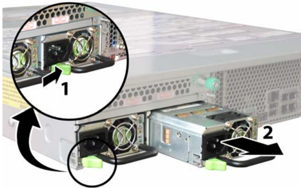
FIGURE 12-12 Removing a Power Supply
