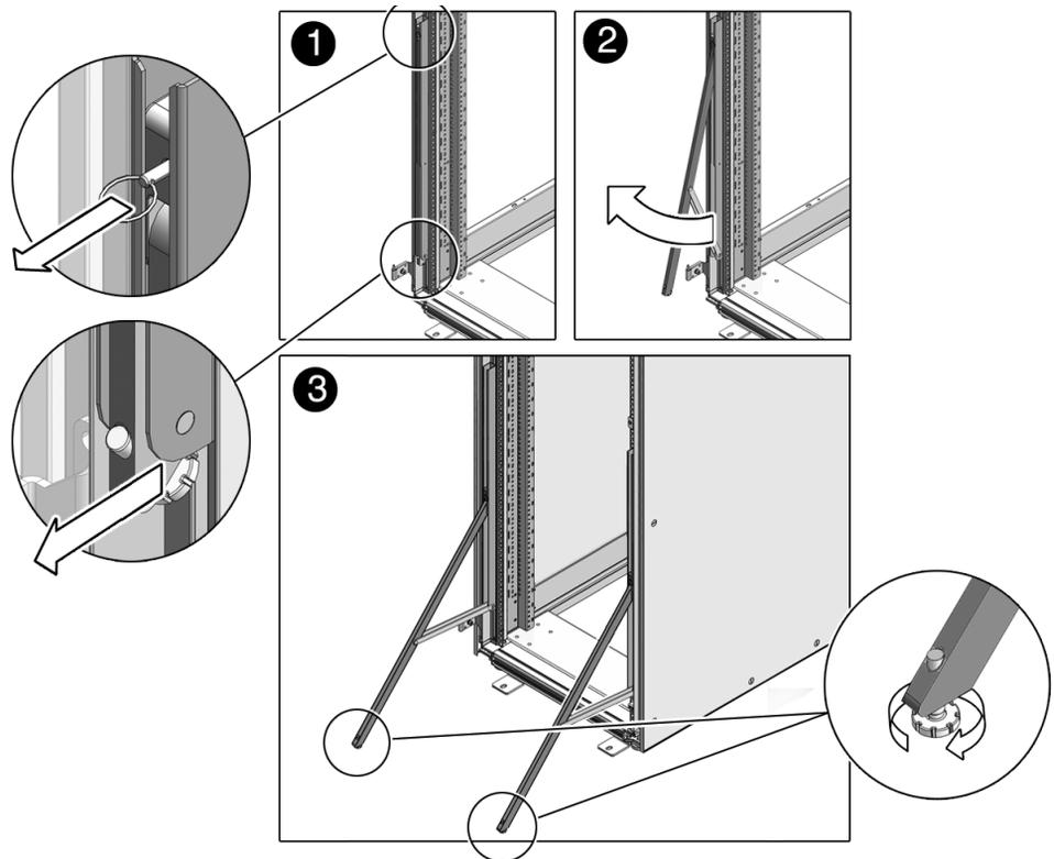
c. Rotate the leg's rubber foot clockwise until it touches the floor (Number 3 in [FIGURE 3-2](#)).
