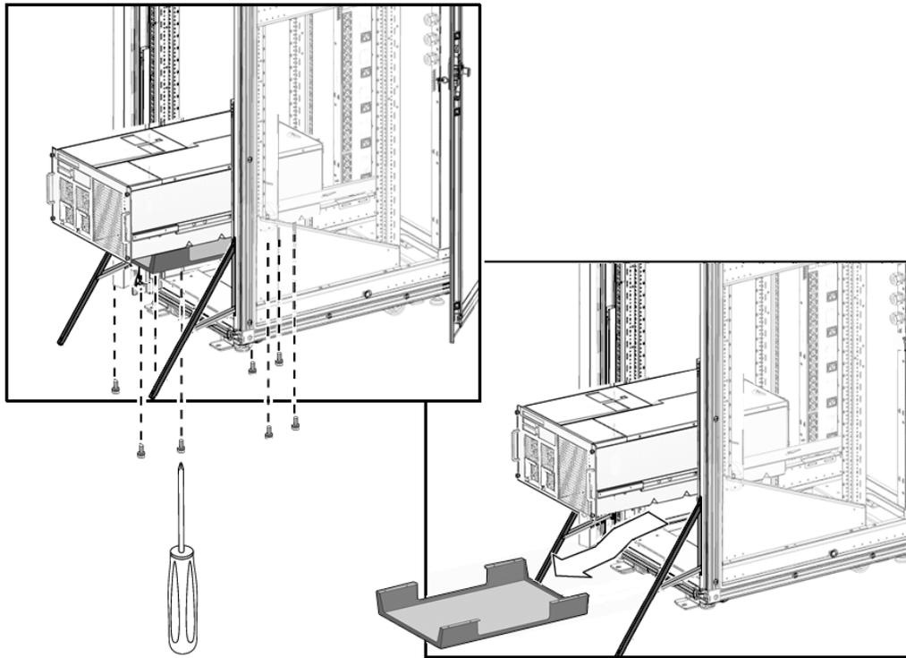
15. Withdraw the computer lifting device.
