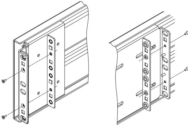
3. Attach four nut bars to the corresponding locations on the ends of the slide rails (front right, front left, rear right, and rear left) with two (2) M2.5 flathead screws at each location.
