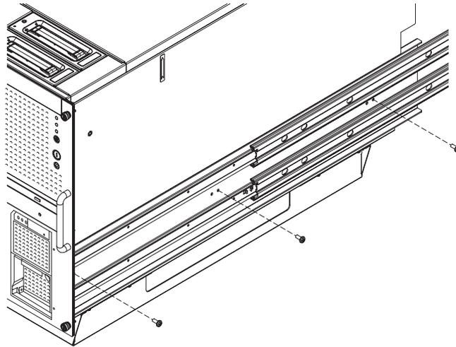
**9. Remove the plinth from the bottom of the server (FIGURE 5-17).**
