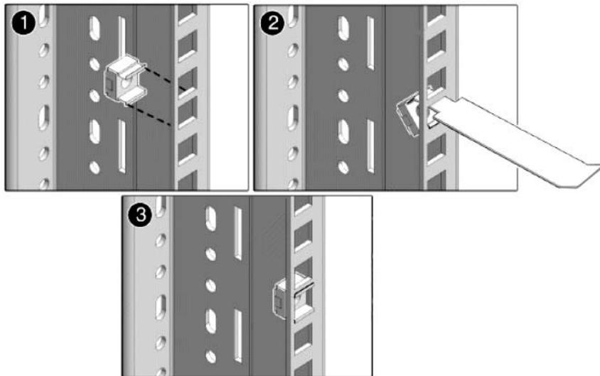
**FIGURE 5-12** Attaching Nut Bars on the M5000 Slide Rail
