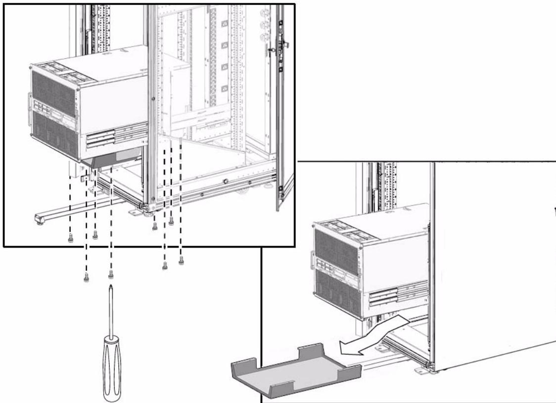
**FIGURE 5-8** Unlocking the M5000 Slide Rail
