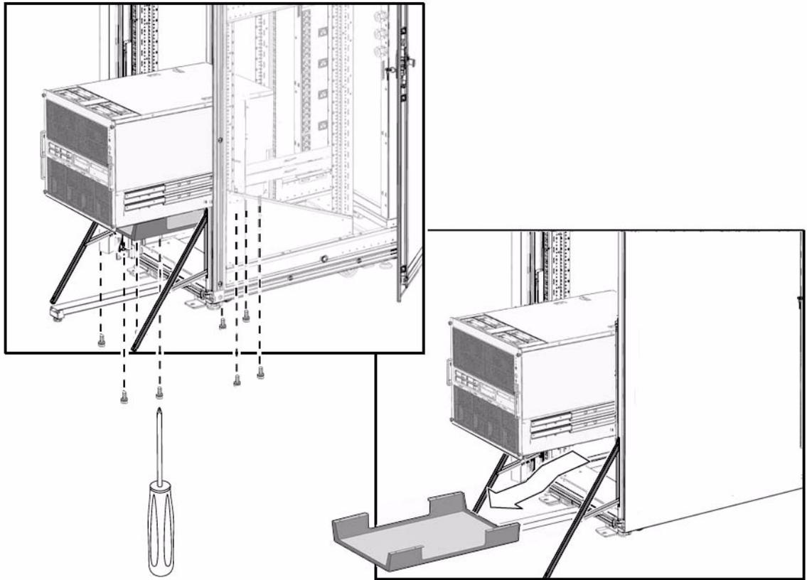
10. Withdraw the computer lifting device.
