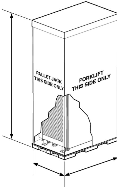
FIGURE 1-4 illustrates the top and front dimensions of a Sun equipment cabinet.
