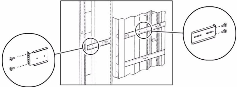
3. Secure the inner parts of the slide rails in place on the server (**FIGURE 4-4**).
