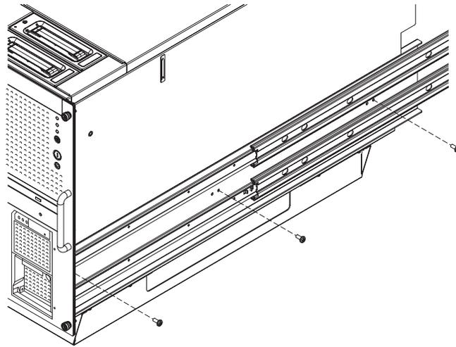
**8. Remove the plinth from the bottom of the server ().**
