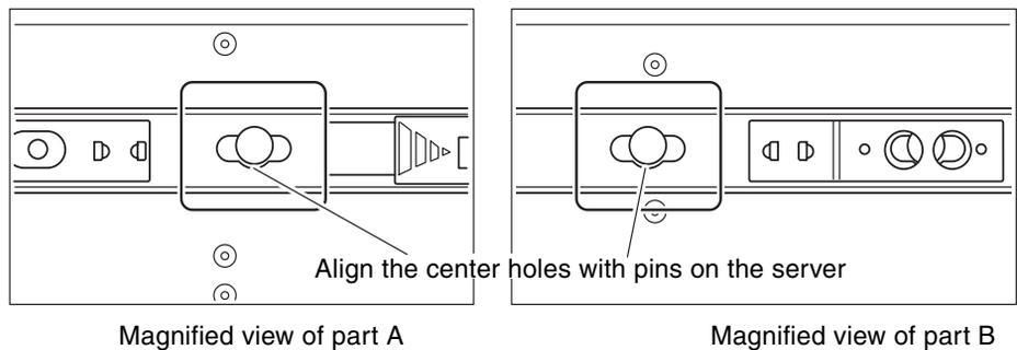
**FIGURE 4-5** Securing Inner Part of the Slide Rail to the Server
