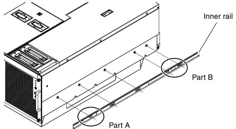
**FIGURE 4-17** Aligning Center Holes With Pins on the Server
