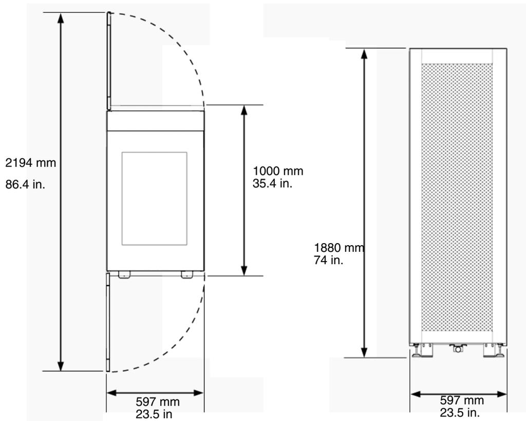
FIGURE 1-5 and FIGURE 1-6 illustrates the footprint of a Sun Rack 1000 and Sun Rack 900.
