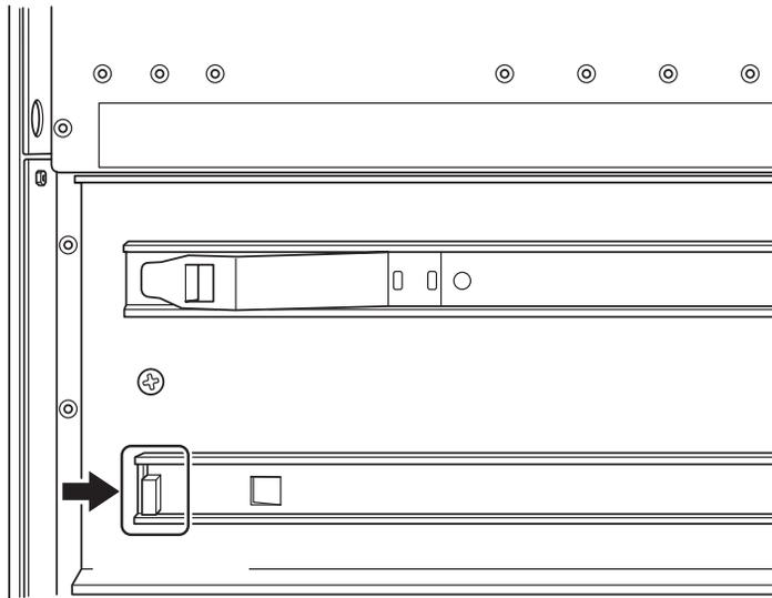
9. **Withdraw the computer lifting device.**
