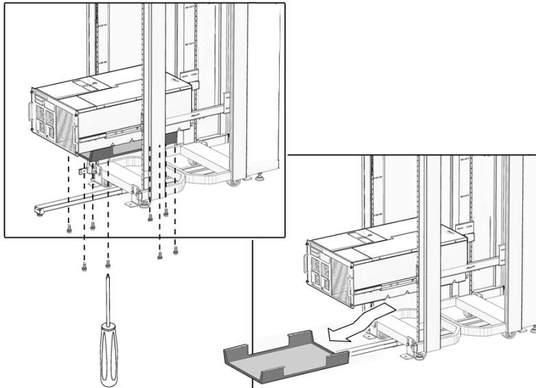
11. Withdraw the computer lifting device.
