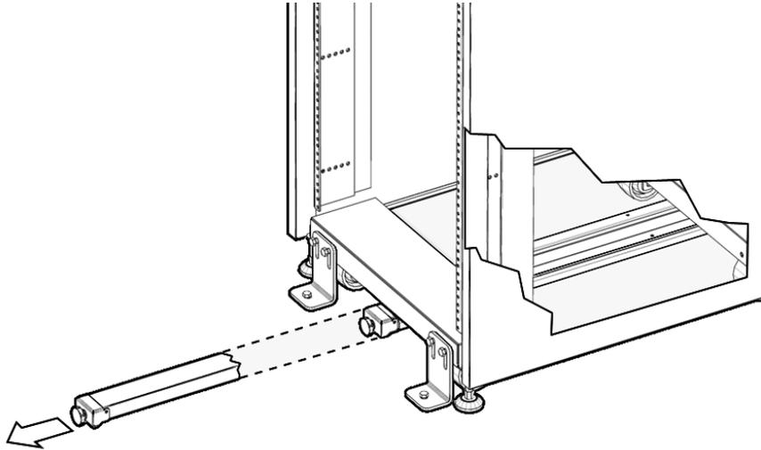
b. Rotate the foot 90 degrees and adjust the height of the foot so that it rests on the floor.
