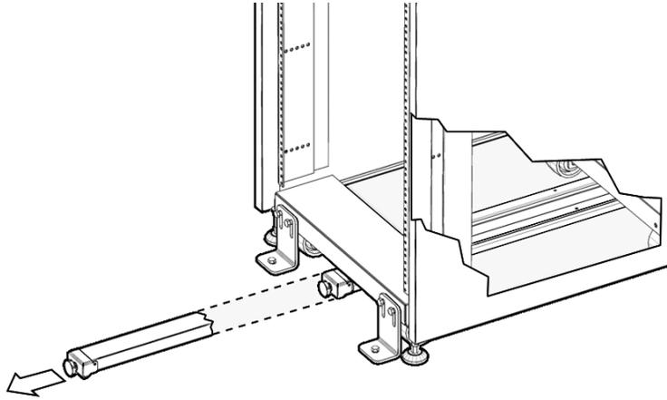
5. Extend the slide rails from the slide assemblies.
