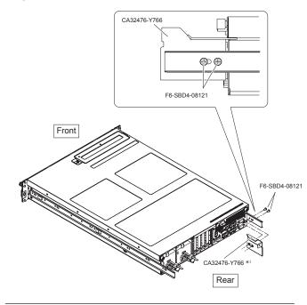
\*1: When replacing or repairing the rail kit, you can use the holding bracket (CA32476-Y766) included in
