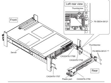
\*1: When replacing or repairing the rail kit only, you can use the screws included in the previous cable management arm kit.
