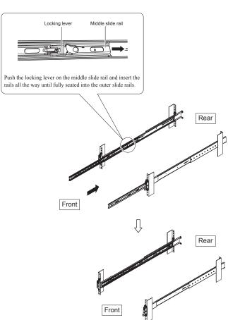
Make sure that the bearing board (thin metal sheet with oval holes) that is housed in the rails is at the front end of the rail.
