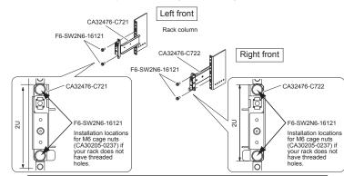
Note - If your rack does not have threaded mounting holes, the mounting screws are secured with M6 cage nuts (CA30205-0237). - 3 -
