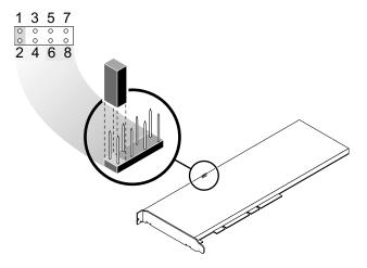
FIGURE G-1 Hardware Jumper Block Pins
