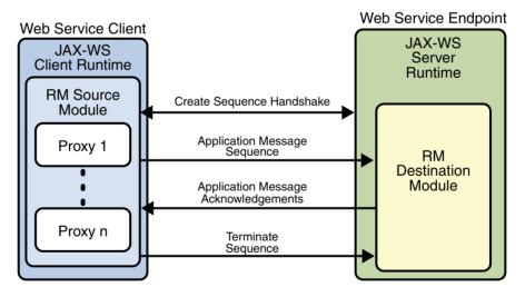
FIGURE 2–8 Application Message Exchange with Reliable Messaging Enabled
