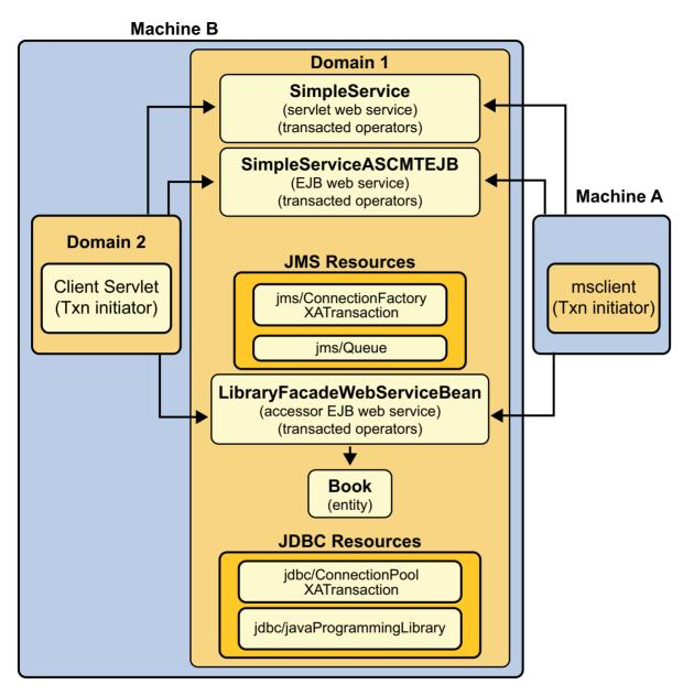
FIGURE 12-2 Components in the basicWSTX Example
