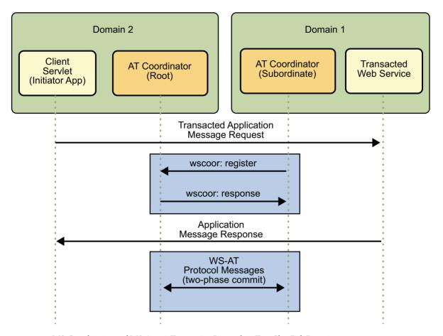
FIGURE 12-1 WS-Coordination and WS-AtomicTransaction Protocols in Two GlassFish Domains
