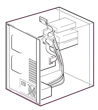
Figure 17 SCSI termination in internal drives
