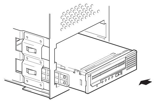
Figure 6 Installing tape drive
