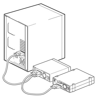
Figure 19 SCSI termination in daisy-chained external drives
