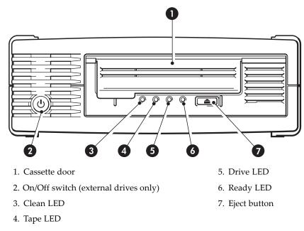
Figure 1 Front view of half-height LTO external tape drive
