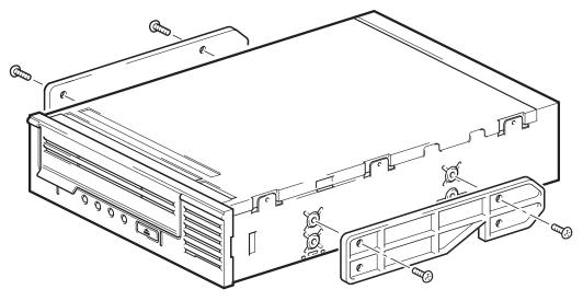
Figure 4 Attaching mounting rails
