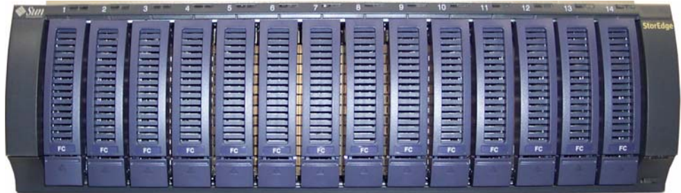
FIGURE 3-4 Sun StorEdge 5300 RAID EU Controller Enclosure Front, With Fibre Channel Disk Drives
