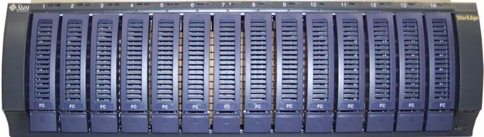
FIGURE 3-6 Sun StorEdge 5300 EU F Expansion Enclosure Front, With Fibre Channel Disk Drives
