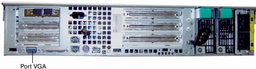
FIGURE 4-5 Port VGA de Sun StorEdge 5310 NAS Appliance
