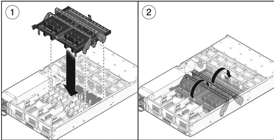
10. Install the memory mezzanine air duct as shown in [FIGURE 2](#).
