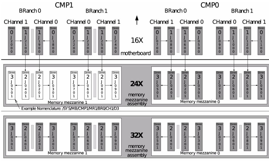
TABLE 1 describes the FB-DIMM FRU names and installation order. Memory mezzanine assembly FB-DIMMs are shaded.
