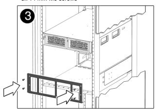
Place the front support bracket into the lower front of the chassis so that the bottom edge of the bracket fits under the chassis and the front of the bracket is flush with the chassis.
