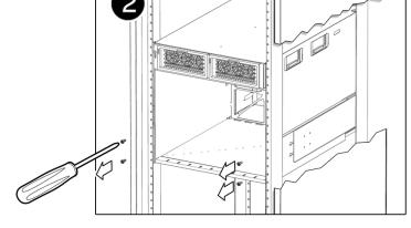
At the front of the system, remove the bottom four screws that fasten the chassis to the rack.
