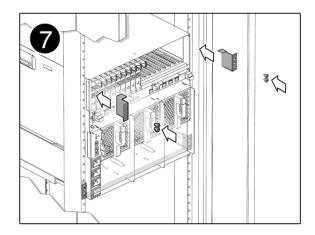
Place the two upper brackets at the top corners of the rear of the chassis.
