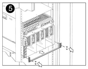
Attach the lower rear bracket so that the lower edge slides under the bottom of the chassis and the middle holes on each side of the bracket fit over the screws protruding from the rack.
