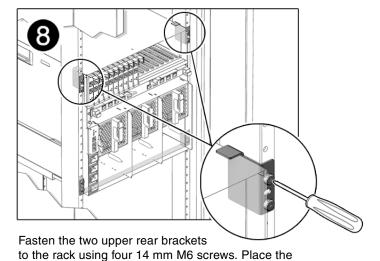
screws in the two outside holes of the bracket, and leave the middle hole empty.
