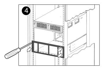
Fasten the front shipping bracket with four 25 mm (or 18 mm) screws. These can be reused to fasten the chassis to the rack when this bracket is later removed.
