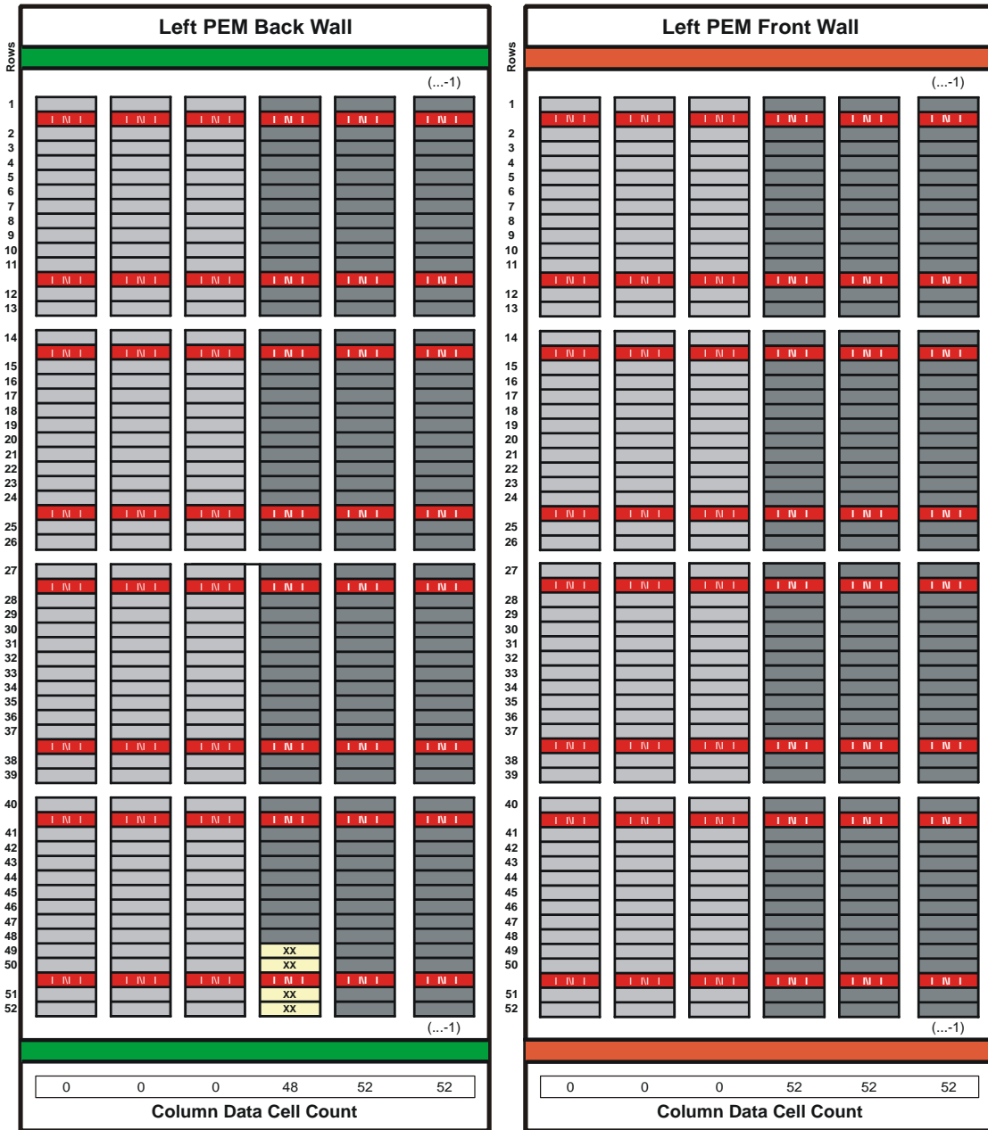
FIGURE A-23 SL3000 Slot Map—Parking Expansion Module, Installed on the Left
