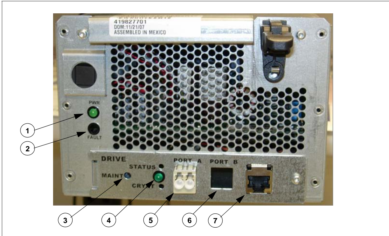
FIGURE 4-2 LTO4 Tape Drive in Drive Tray—SL8500
