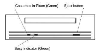
Cassettes in place indicator - Lit when a tape is in the drive Drive busy indicator - Flashes while data is being written to/read from the drive Eject button - Used to eject the tape
