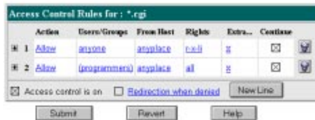
Figure 6.8 Restricting access to a file type—in this case, to files with the .cgi extension
