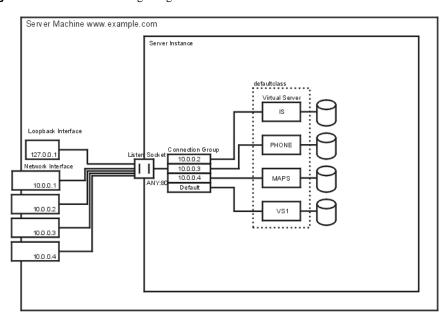
**Figure 13-6** Intranet hosting using IP-addressed-based virtual servers
