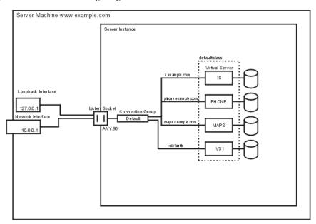
Figure 13-5 Intranet hosting using URL-host-based virtual servers
