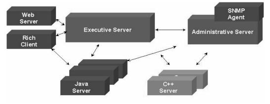
When a web server forwards requests to iAS, the requests are first received by the Executive Server process (KXS). The KXS process forwards the request either to a Java Server process (KJS). A KJS process runs Java programming logic. Note that for migration purposes a KCS, C++ engine exists and runs C++ programming logic. KCS runs in a similar manner to the KJS engine.
