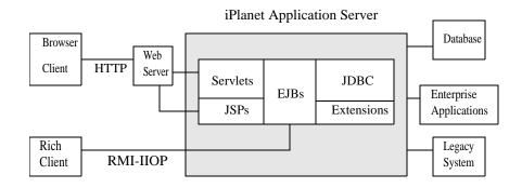
The Rich Client is a first-tier program that executes in its own Java Virtual Machine (JVM), possibly in an ACC. Deploying the Rich Client requires the specification of deployment descriptors using XML.
