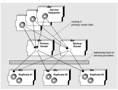
Figure 6-8 Load Balancing Scheme with Failover
