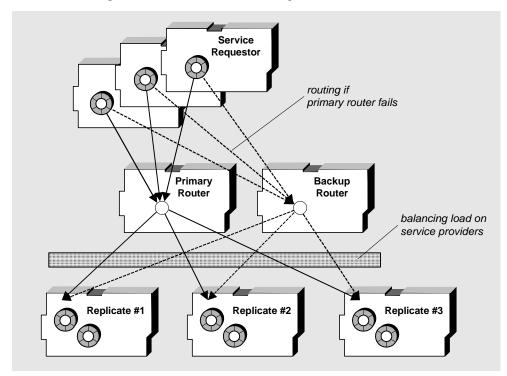
Figure 1-7 Replicated Partitions: Load Balancing and Failover
