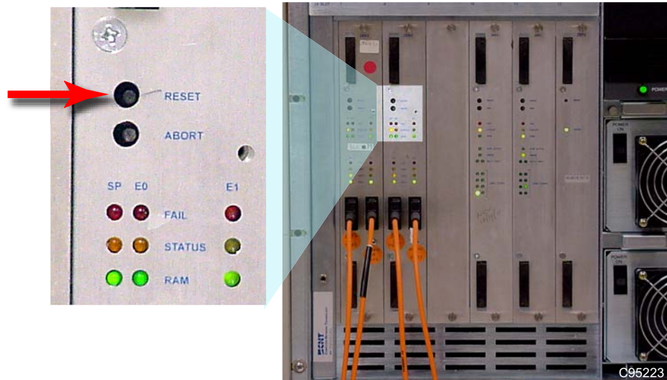
Figure 33 CNT Interface Card Reset Button Location
