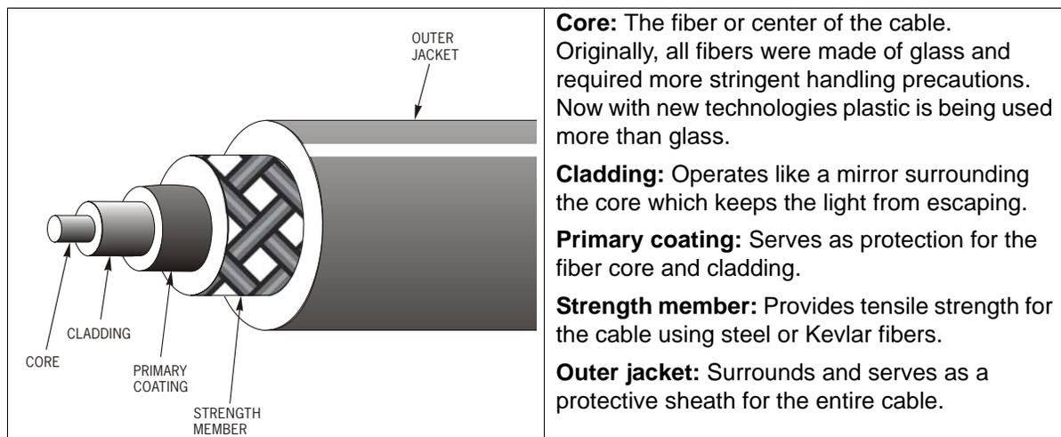
**Core:** The fiber or center of the cable. Originally, all fibers were made of glass and required more stringent handling precautions. Now with new technologies plastic is being used more than glass.
