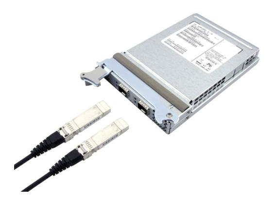
2. Insert the other end of the copper cable, or cables, into an empty SFP+ cage on the FCoE switch.
