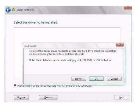
a. Ensure the storage driver(s) are accessible according to the installation method chosen (described in Appendix A).
