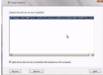
d. In the Select the Driver to Be Installed dialog, click  $\mathtt{Next}$  to install the driver.
