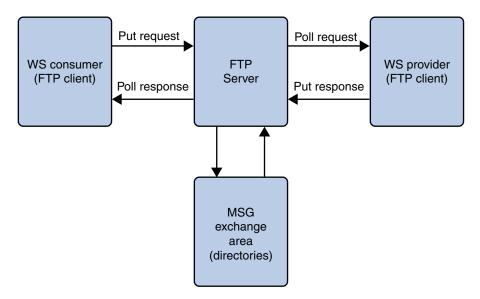
The figure illustrates a full message path including request (IN-ROUTE) and response (OUT-ROUTE). As illustrated, FTP Binding Component uses directories on FTP server as message persistence where service consumers and service providers exchange messages. During the implementation the following assumptions are made to facilitate message transportation in a FTP context.
