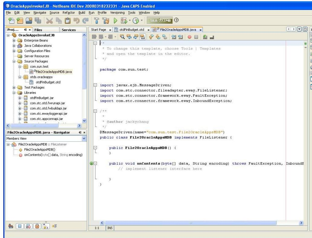
17 In the generated MDB, drag Oracle Applications from the palette to invoke Oracle Applications.
