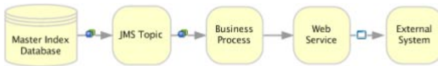
FIGURE 3 Outbound Message Processing Data Flow
