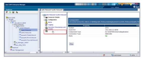
8 Terminate the external system and observe that the status information of the terminated system no longer appears in the status table
