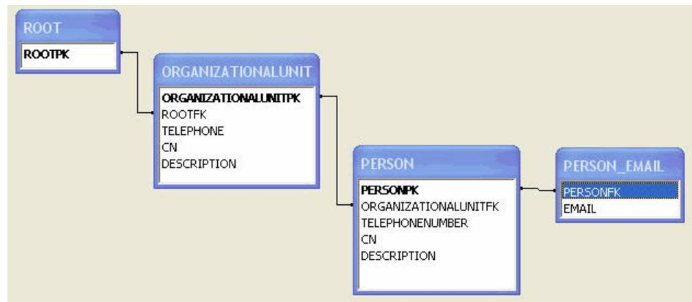
This graphic shows the relational structure created by the LDAP to relational mapping process from the LDAP tree example.
