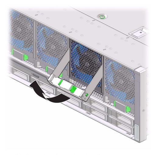
6. Pull the fan module out from the chassis by the lever.
