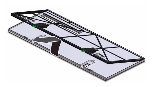
9. Lift the air filter out of the filter tray and set it aside.
