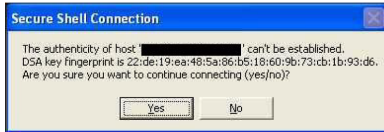
Figure 4-2 Initial SSH Connection Window
