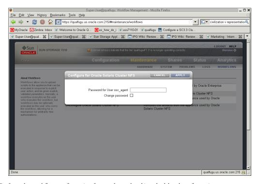
Perform the workflow configuration from only one head in a dual-head configuration.
