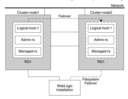
FIGURE 1-2 Oracle Solaris Cluster HA for WebLogic Server File System Failover Configuration
