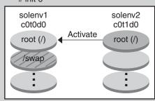
2 Upgrade an inactive boot environment. For a standard upgrade: (a) # luupgrade -u -n solenv2 \ -s /net/installmachine/export/Solaris/OS\_image solenv1 solenv2 c0t0d0 c0t1d0 Upgrade root (/) root (/) swap Release Y For a Solaris Flash archive: (b) # luupgrade -f -n solenv2 \ -s /net/installmachine/export/Solaris/Release\_Y \ -a /net/server/archive/Release\_Y solenv1 solenv2 c0t0d0 c0t1d0 root (/) root (/) Solaris Release Flash swap Υ archive
