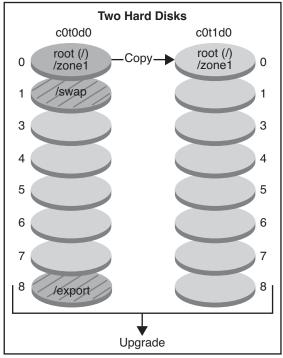
Single disk command: # lucreate -c bootenv1 \ -m /:/dev/dsk/c0t0d0s4:ufs \ -n bootenv2 Two disks command: # lucreate -c bootenv1 \ -m /:/dev/dsk/c0t1d0s0:ufs \ -n bootenv2
