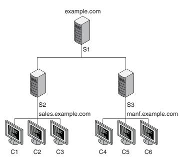
Clients C1, C2, and C3 would obtain their network information from server S2. Clients C4, C5, and C6 would obtain information from server S3. The resulting network is summarized in the following table. The table is a generalized representation of that network but does not resemble an actual network information map.
